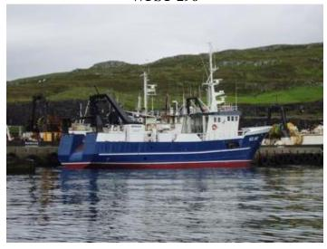
**Type** Wet fish stern trawler, with wheelhouse forward.
